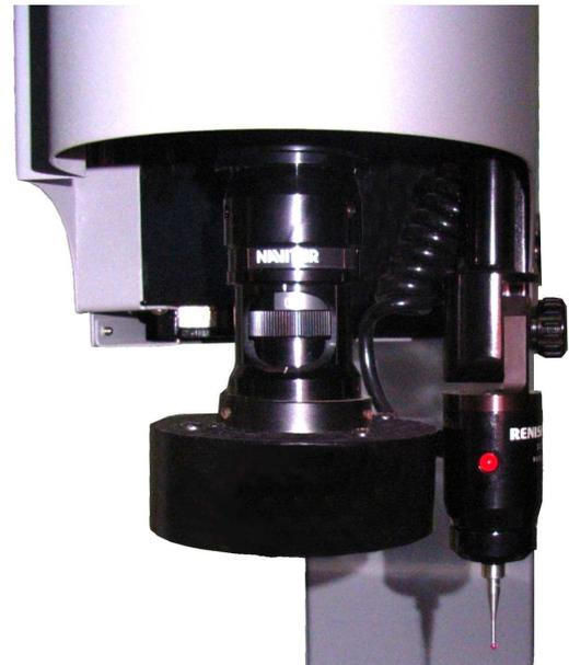
■ Powerful zoom lens with high resolution linear encoder to provide accurate micro image inspection for precision parts.
