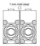
Figure 2.1 Side-by-side mounting of STAs must be separated by a 1 mm thick mild steel plate
