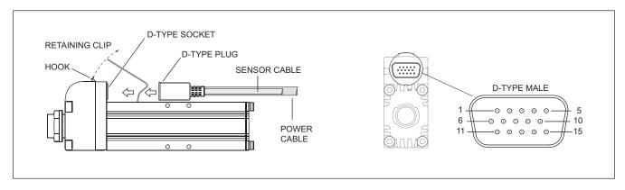
Figure C.3 Shows connecting the cable assembly to the forcer and connector details
