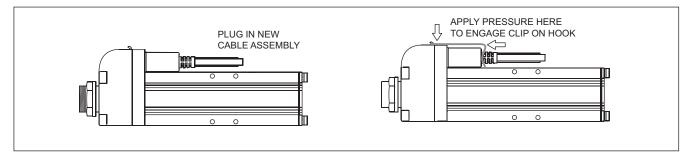
Figure 3.2 (left) Plugging in the new cable assembly and (right) fitting the retaining clip.
