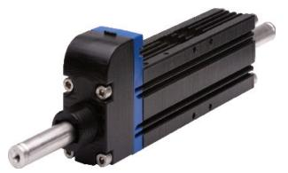
The patented magnetic design of ServoTube generates 12 micron (0.47 mil) repeatability and 350 micron (14 mil) accuracy from a non-contact, integral position sensor. No external encoder is required. Position output is industry standard 1V pk-pk sin/cos signals.
