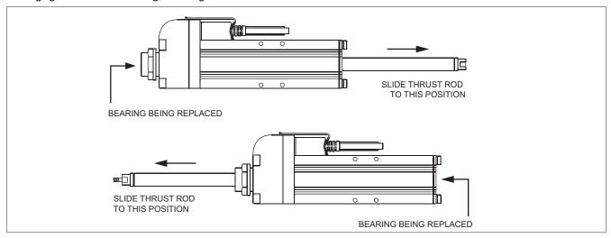
Figure 3.3 Positioning the thrust rod when removing a bearing.
