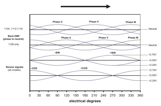
Figure C.1- The relationships between motor phase back EMF and position sensor outputs
