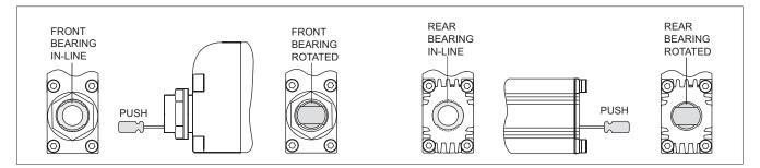
Figure 3.4 Setting the orientation of the front (left) and rear (right) spherical bearings.
