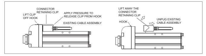
Figure 3.1 (left) Removing the retaining clip and (right) removing the cable assembly.
