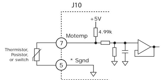
\* Alternate Sgnd connections on J10 are pins 16, 25, 26
