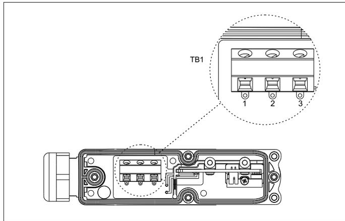
Figure C.3 - Power cable connection at TB1
