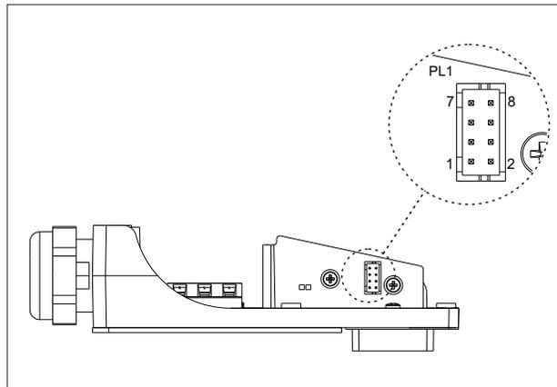
Figure C.4 - Sensor cable connection at PL1 on the Sensor PCB
