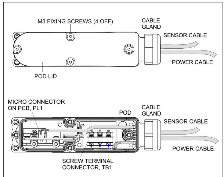
Figure 3.1 - Power and Sensor cable connection details in the pod
