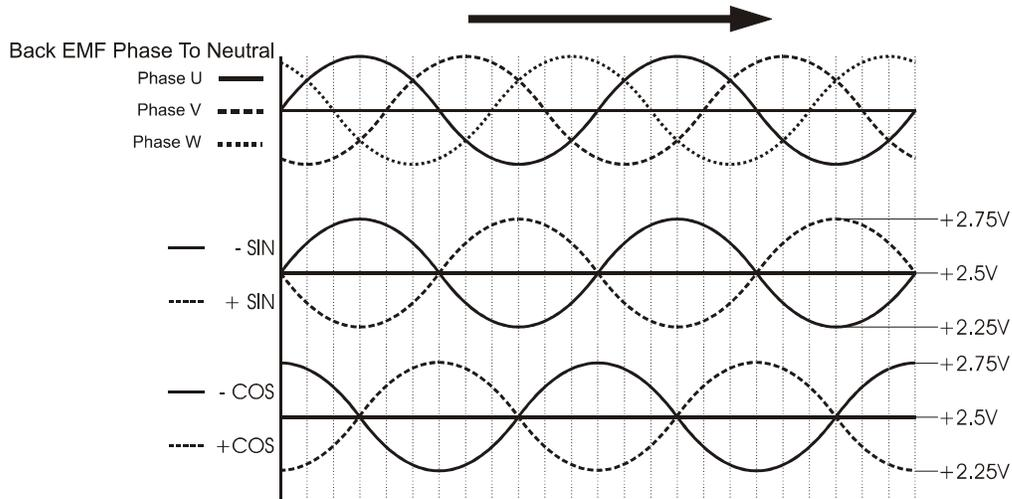
Figure C.3- The relationships between motor phase back EMF and position sensor outputs
