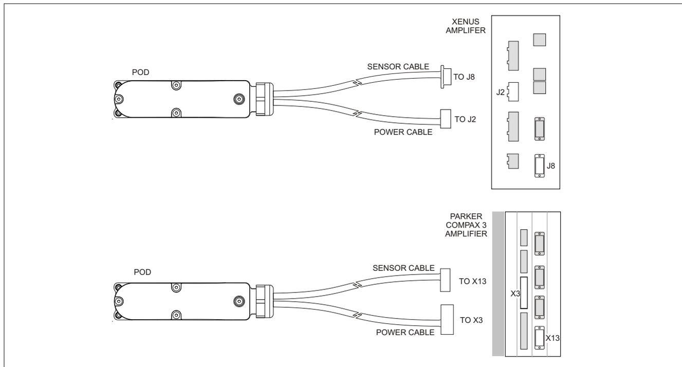
Figure 2.2 - Schematic showing connection of the XTR25 to the Xenus Amplifier and Parker Compax 3 Amplifier
