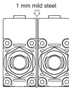
*Figure 2.1 Side-by-side mounting of STAs must be separated by a 1 mm thick mild steel plate*
