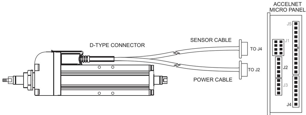
*Figure 2.3 - Schematic showing connection of STA / STB to the Accelnet Micro Panel Amplifier*
