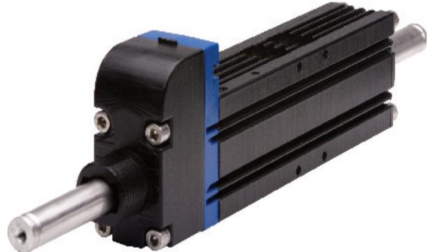
The patented magnetic design of ServoTube generates 12 micron (0.47 mil) repeatability and 350 micron (14 mil) accuracy from a non-contact, integral position sensor. No external encoder is required. Position output is industry standard 1V pk-pk sin/cos signals.
