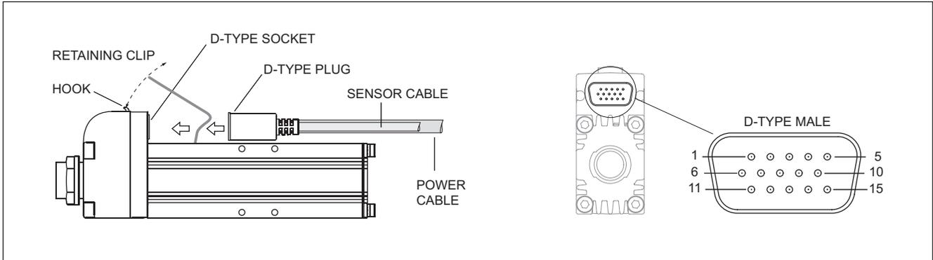
Figure C.3 Shows connecting the cable assembly to the forcer and connector details
