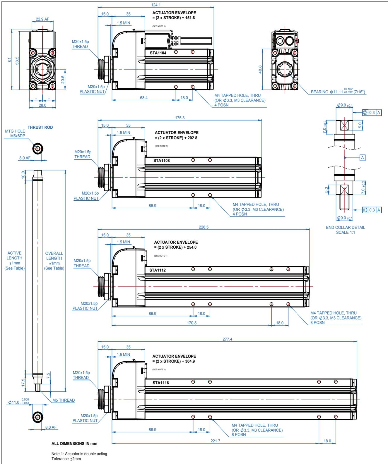
Figure 2.1 STA outline drawings and mounting details
