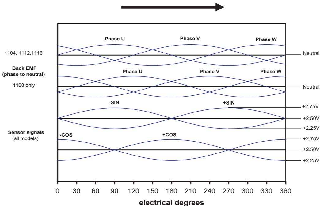
Figure C.1- The relationships between motor phase back EMF and position sensor outputs
