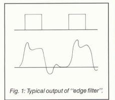
the voltage waveforms from the amplifier. An edge filter is designed to operate on the voltage transitions or edges or the voltage waveforms as shown in (Fig. 1)
