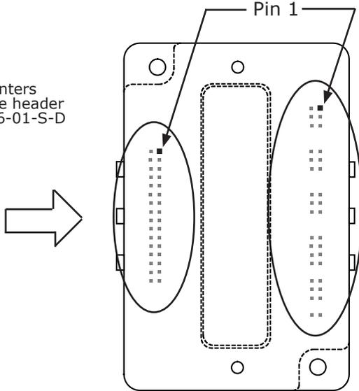
Drive viewed from above looking down on the pc board on which it is mounted. Pins and housing shapes are shown in phantom view.
