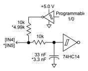
\* [IN5] connects to J2 for motor overtemp switch
