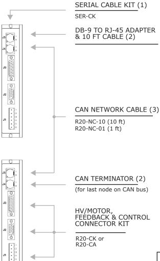
Multiple drives are connected as nodes on a CAN bus
