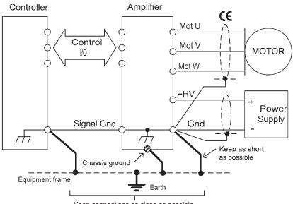
Keep connections as close as possible. "Star" ground to a common point is best
