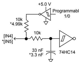
\* [IN5] connects to J2 for motor overtemp switch
