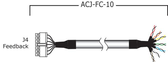
This cable plugs into drive J4 and consists of seven twisted-pairs of AWG 24 wire. Each pair has a black and colored conductor. The chart above shows twisted-pairs in the rows. E.g. one pair goes to pins 1&8, another pair to pins 2&9, etc. Cable termination is flying leads for connection to customer motor feedback encoder.
