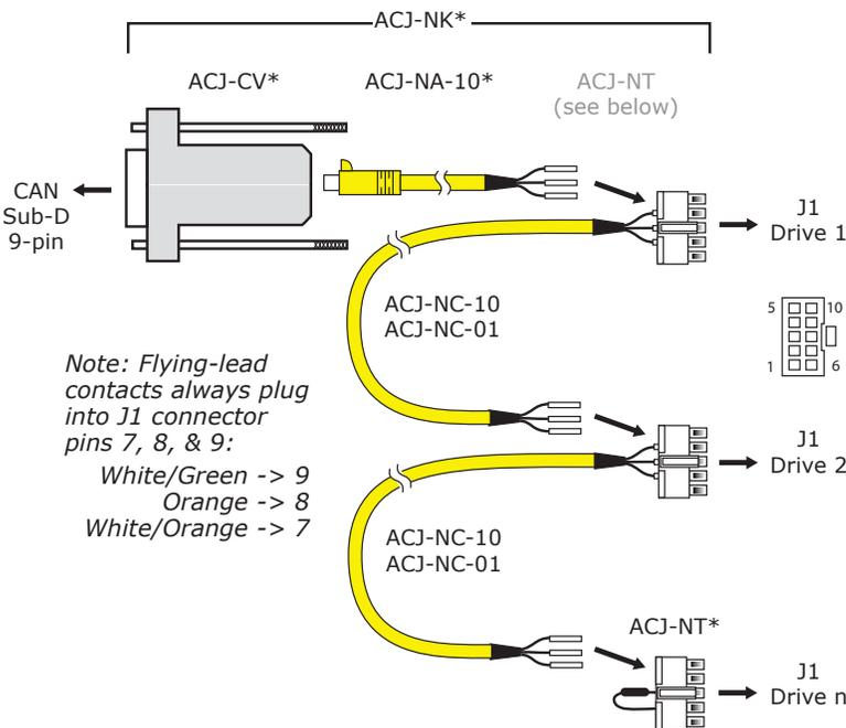
Note: Flying-lead contacts always plug into J1 connector pins 7, 8, & 9:
