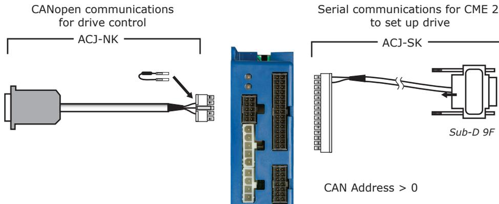
MULTIPLE-DRIVE SETUP FOR CANOPEN POSITION CONTROL
