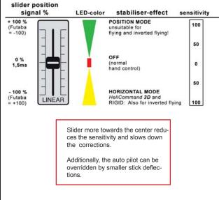
You may of course exchange up with down side, by reversing transmitter setting or slider mounting. Tail rotor gyro
